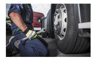
Pressure checks can be combined with regular visual inspection to identify wear problems due to poor alignment. This doesn't require expensive equipment – just a pressure gauge and the commitment to do it. Moving beyond human-based systems to a tyre pressure monitoring system (TPMS) or automatic inflation system is covered in the Get Fleet Fit Efficiency Upgrades fact sheet.
